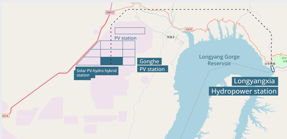
Operation of hydropower and PV generation under one joint control system at the hybrid facility makes it possible to provide immediate compensation between both technologies and adjust the output power to the power grid's needs. This means the efficiency of both technologies is increased, reducing curtailment and boosting revenues.
